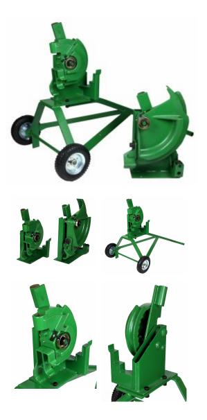
Toledo Pipe Tools is proud to give you an alternative quality Mechanical Conduit Bender. The 1800 Ratchet Bender is a manually powered bender intended to bend 1/2", 3/4", 1", 1-1/4" and 1-1/2" IMC (intermediate metallic conduit), Rigid Conduit and Schedule 40 Pipe. It comes with two heads the 1800 head for 1/2", 3/4", and 1". The other 1801 head for 1-1/4" and 1-1/2".
