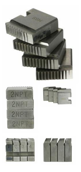
PRODUCT DESCRIPTION Toledo Pipe Tools is proud to give you an alternative quality pipe threading replacment dies. These dies are made from quality high speed steel and are machined to work with RIDGID® 12R, 00R, 11R, 0R Die Heads. The application of these replacement dies are for Right Hand NPT.
